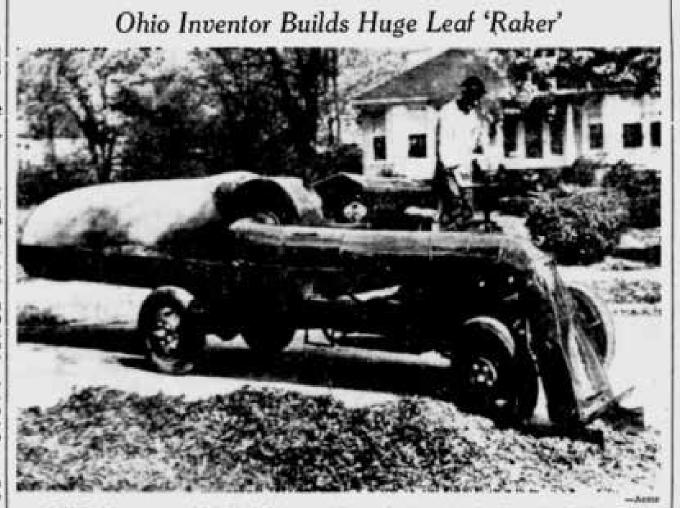
A LEAF picker-upper which Fred Gedge, public service impector for Wyoming, Ohio, thought up is shown in operation. He took an old truck, ready for the scrap heap, mounted on it an equally old motor from another auto, attached a second hand fan and some pipe and this is the result.
